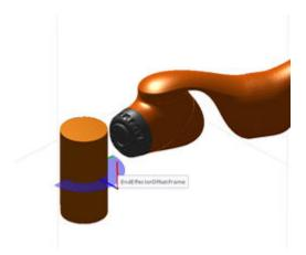
The object is typically used with rapidly exploring random tree (RRT) planners like the manipulatorRRT object. Specify your workspace goal region as the third input to the plan function. Using the workspaceGoalRegion object, the planner can plan to multiple reachable goal endeffector poses during planning and give collision-free paths.
